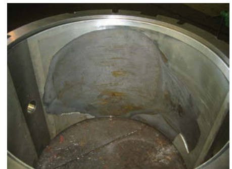
FIGURE 1 (TOP LEFT) AND ABOVE: Sterntube bearing white metal damage
